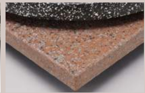
260 1 1/4" Eased Flat Edge. 1/8" veneer solid surface material over a 3/4" exterior grade plywood core.
